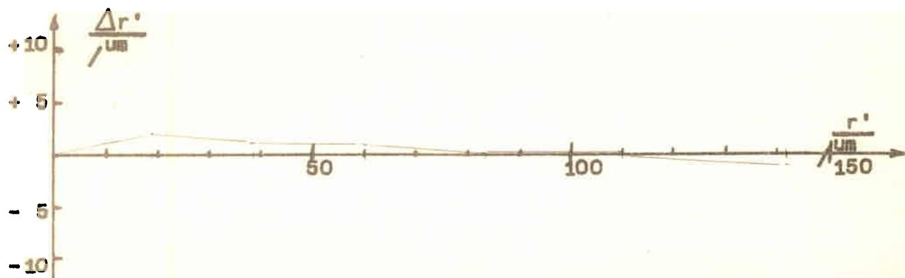
**Distortion on the semidiagonals related to the symmetry point of distortion**
