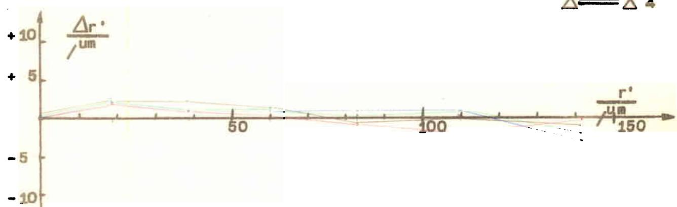
**2.5. Tangential residual errors****Mean value for the largest field angle**Diagonal 1 - 2:  $\pm 2 \mu\text{m}$ Diagonal 3 - 4:  $\pm 1 \mu\text{m}$ **3. Image coordinates of the fiducial marks (mm)**
