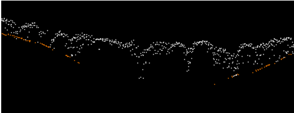
Figure 3. In very rough terrain, the ground surface generally becomes difficult to define, especially with low point density. As the terrain model is being produced based on laser points classified as ground, this type of mountain slopes may entail major local errors in the terrain model. Photo: Andreas Rönnerberg
