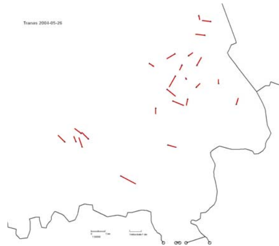
Figure 5: The residuals after transformation of control points with RIX 95 transformation parameters.
