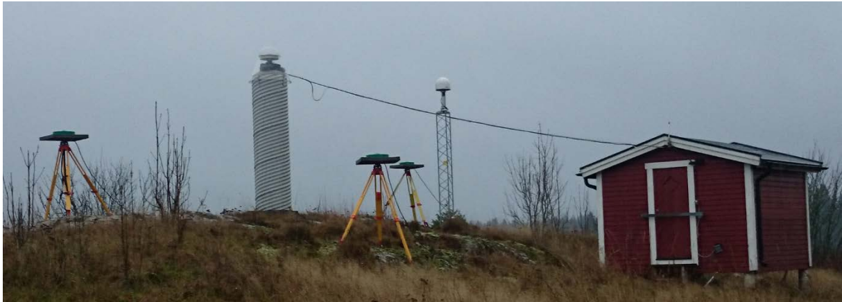
Figure 2. The SWEPOS site Vänersborg during a station calibration setup in November 2014. An Eccosorb plate is mounted directly below the choke-ring antenna. Note the typical SWEPOS concrete pillar and the recent steel-grid mast with the LEIAR25.R3 antenna and LEIT radome installed.
