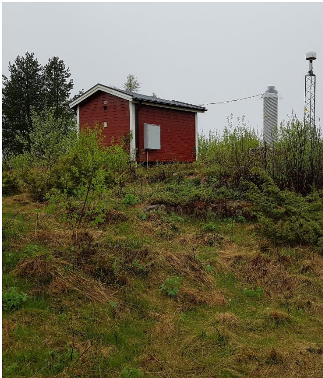
Figure 3: Sveg is a SWEPOS class A station. It has both a new monument (established in 2011) and an old monument (from 1993).
