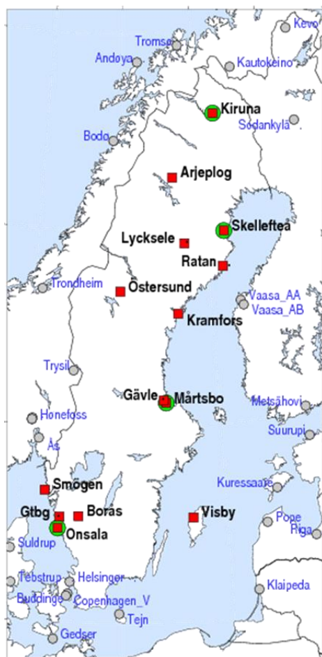
Figure 7: There are 14 absolute gravity sites (for FG5/FG5X) in Sweden marked with red squares in the map. Absolute gravity sites in neighbouring countries are marked with grey circles. The four sites with time series more than 15 years long have a green circle as background to the red square.
