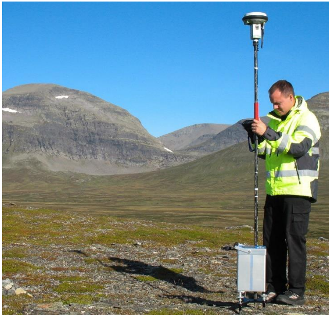
Figure 6: More than 3,400 new relative gravity measurements have been performed in Sweden since 2010. The heights of the locations are determined by network RTK measurements. Photo: Örjan Josefsson.
