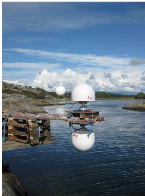
Figure 3.4: GNSS-based tide-gauge at the Onsala Space Observatory.
